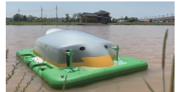
The Aigamo Robot operating in a rice paddy
